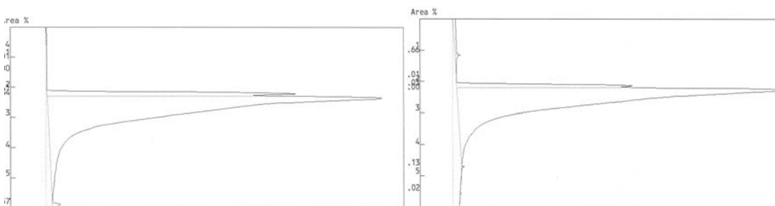
Figure 6. Left GC diagram of solvent G-0028 before distillation Right GC diagram of solvent G-0028 after distillation
